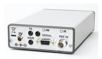
The 409B is a 171 MHz, Four Channel, Direct Digtal Synthesized Signal Generator in a small table top case. The 409B generates four output signals simultaneously up to 171 MHz in 0.1Hz steps under serial control. The frequencies of the four outputs can be independently set and can be offset from each other by 14-bits (0.02°) of programmable phase. The sine wave amplitudes are 10-bit programmable.
