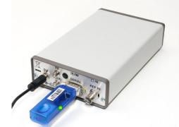
or tablet. The wireless communication range is approximately 30 feet. A solid green light on the DB9 dongle shown above indicates a successful wireless connection. The USB Dongle uses the FTDI chipset. Most computers will automatically set up a virtual COM port when the USB dongle is plugged in. The USB dongle has been used successfully with Android devices running the "Serial USB Terminal" Android application, available from Google Play.
